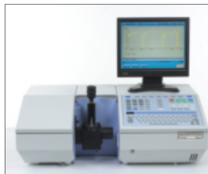
Figure 1. Spectrum RX I with single reflectance ATR.
