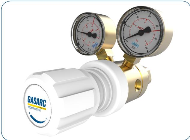
The Tech Master GPT410 Series two stage diaphragm cylinder regulators are designed for primary pressure gas control of technical grade Acetylene gas up to 4.5 purity (99.995%), on applications where constant delivery pressure is required as the cylinder pressure decreases.
