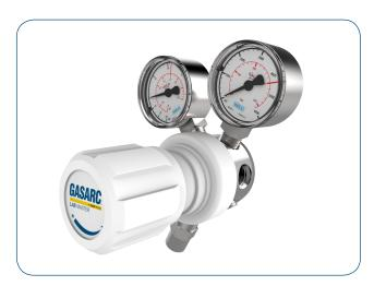
The Lab Master LGS500 Series single stage diaphragm cylinder regulators are designed for primary pressure gas control of non-corrosive or toxic, high purity gases up to grade 5.0 purity (99.999%), on applications where slight variation from decreasing cylinder pressure is acceptable.
