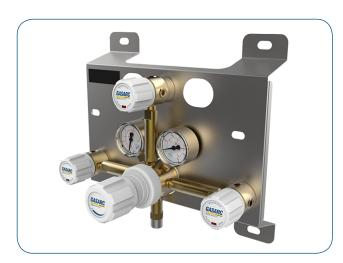
The Tech Master GPM4040 Series two stage twin cylinder manual change control panels are designed for primary pressure gas control of non-corrosive or toxic, technical gases up to grade 4.5 purity (99.995%), on gas distribution systems where constant delivery pressure is required.
