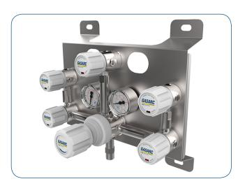
The Lab Master LGM5040 Series two stage twin cylinder manual change control panels are designed for primary pressure gas control of non-corrosive or toxic, high purity gases up to grade 5.0 purity (99.999%), on gas distribution systems where constant delivery pressure is required.
