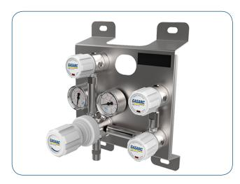
The Lab Master LGM5020 Series two stage single cylinder manual change control panels are designed for primary pressure gas control of non-corrosive or toxic, high purity gases up to grade 5.0 purity (99.999%), on gas distribution systems where constant delivery pressure is required.
