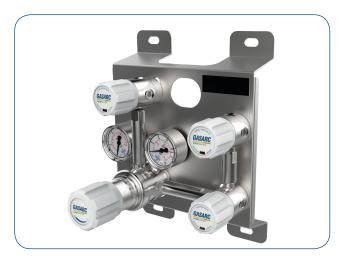
The Chem Master SGM6020 Series two stage single cylinder manual change control panels for primary pressure gas control of corrosive, toxic or high purity gases up to grade 6.0 purity (99.9999%), on gas distribution systems where constant delivery pressure is required.
